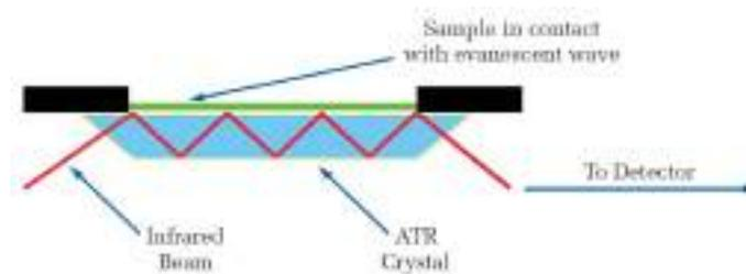
**Figure 2 :** Working of diamond ATR in FTIR spectrometer
