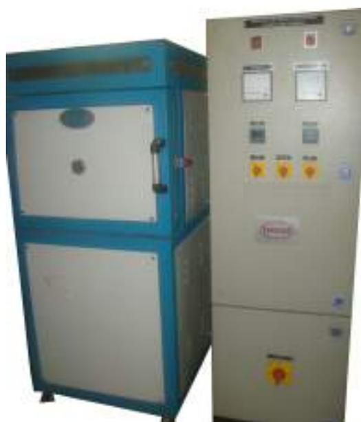
**Figure 3:** High temperature conventional resistive furnace
