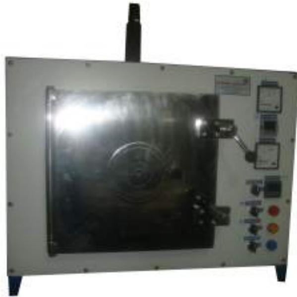
**Figure 5:** High temperature resistive coupled microwave furnace
