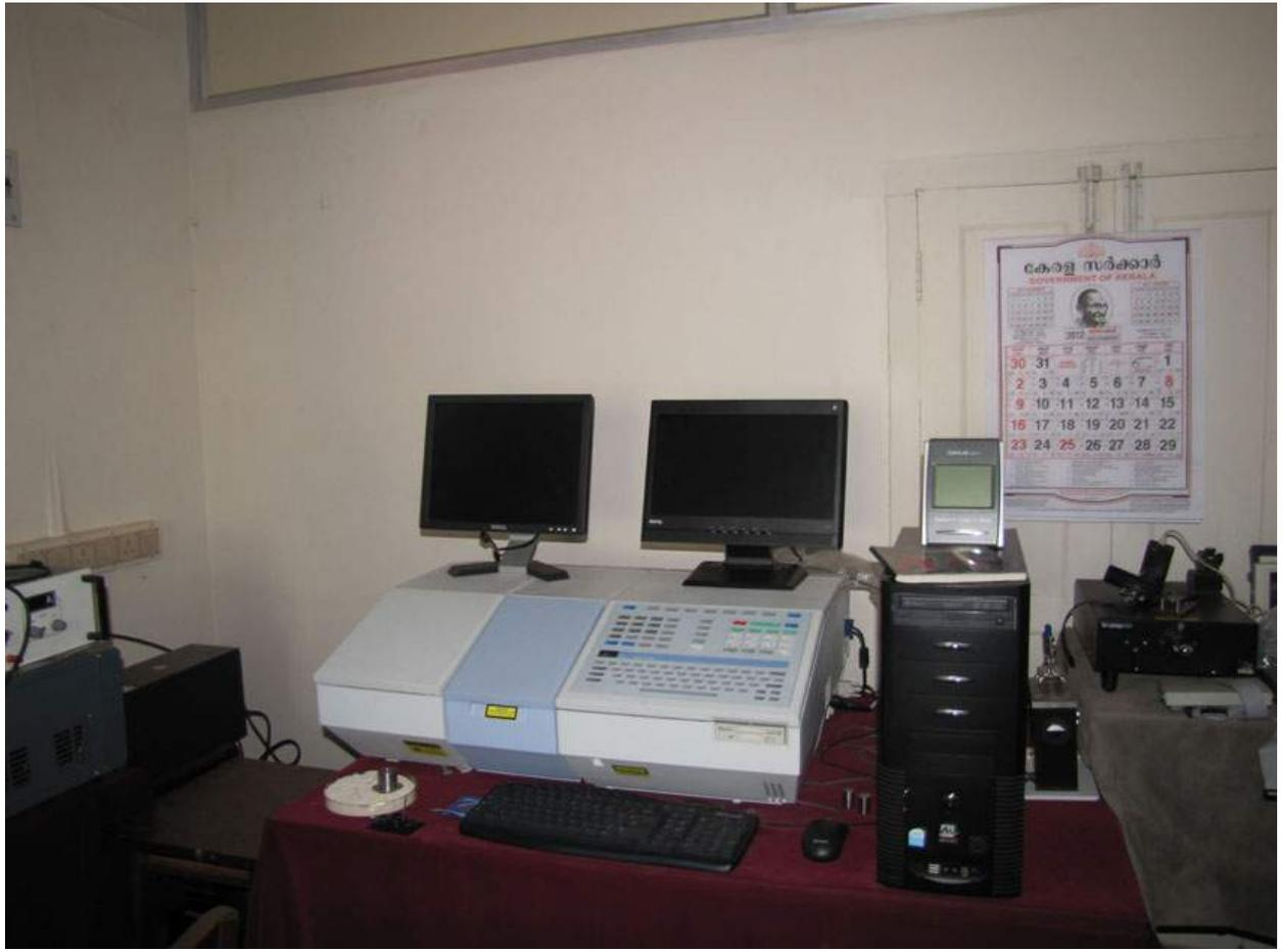
Perkin Elmer IR Spectrometer
