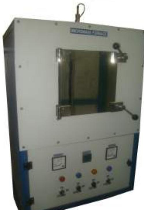
**Figure 4:** High temperature susceptor assisted microwave furnace
