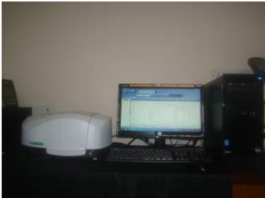
**Figure 1 :** Perkin Elmer Spectrum two with diamond ATR accessory
